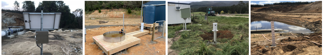
Logging and telemetry of flow meters, rainfall, evaporation and dam level
